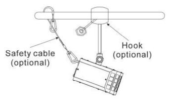
use a safety cable that can hold 12 times of the weight of the unit when installing the fixture. The equipment must be fixed by professionals. And it must be fixed at a place where is out of the touch of people and has no one pass by or under it.
