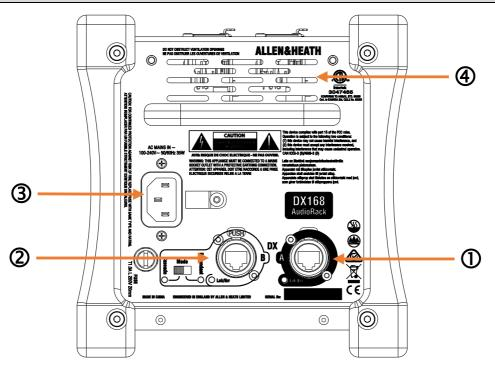
**DXA** EtherCon port for connection to the mixing system. The cable carries the audio signals as well as preamp control and system status data.
