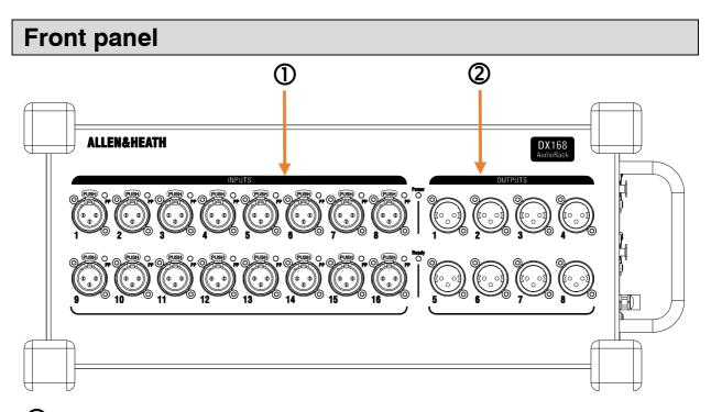
0 Input sockets Balanced XLR mic/line inputs with +48V Phantom Power indicator. The preamps are built into the DX168 and their Gain, Pad and +48V are controlled from the mixer via the DX link.
