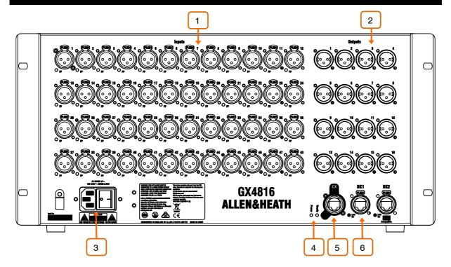
Input sockets – Balanced XLR mic/line inputs with +48V Phantom Power indicator. The preamps are built into the GX4816 and their Gain, Pad and +48V are controlled from the mixer via the Cat5 link.
