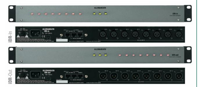
iDR-8 and iDR-4 can happily manage many complete systems with their existing input/output architecture standing alone. However, for larger systems, iDR-In and iDR-Out audio expander units are available, providing an additional 8 mic/line inputs on XLR and 8 line outputs (also on XLR) respectively. One or both expanders may be connected to a single iDR main unit.
