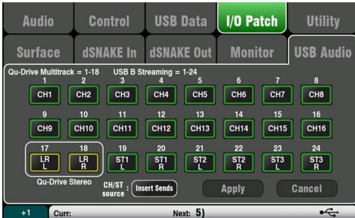
Toggle the CH/ST source from 'Insert Send' to 'Direct Outs' and press 'Apply'.
