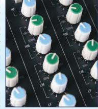
frequencies below 80Hz. HM and LM are bell shaped peak/dip filters which affect frequencies around a centre point which can be swept from 500Hz to 15kHz and 35Hz to 1kHz respectively. These have a width (Q) of 1.8. All bands can be boosted or cut by up to 15dB and have a centre detent 0dB position. EQ In/Out switching makes it easy to compare the sound with the equaliser switched in or out of the circuit.
