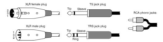
The input and output **XLR** connectors are 3 wire differentially balanced. These have 3 connector pins: Pin 1 = ground (screen), Pin 2 = signal hot (+), Pin 3 = signal cold (-).
