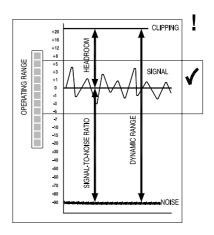
The diagram above illustrates the operating range of the audio signal.
