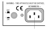
4 Connect AC mains power. Check first that the correct mains lead with sealed plug suitable for your local supply has been provided with your console. Plug into the AC MAINS IN socket making sure the connector is pressed fully in.
