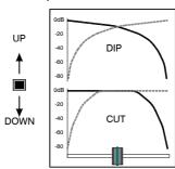
**XFADE ON**. In the up position the music signal is routed directly to the mix. Press to route the signal through the crossfader.
