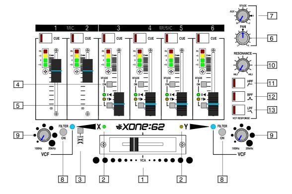
1 VCA Crossfader. The XONE:62 uses four high performance voltage controlled amplifiers (VCA), a pair for each side of the stereo crossfader. The robust 45mm fader produces a DC control voltage which determines the signal level of the VCAs. The voltage is filtered to prevent any audible noise, clicks or scratchiness resulting should the fader track become worn. This benefit would not be possible if the signal were routed through a conventional audio fader.
