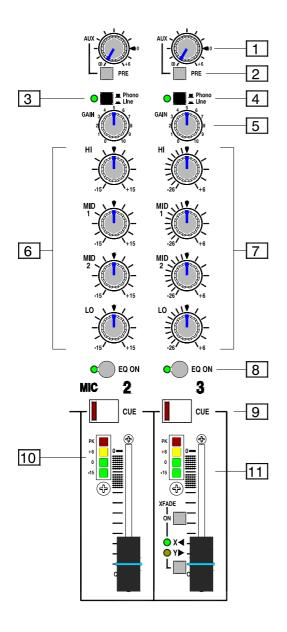
1 AUX send. Adjusts the level of the channel signal to the stereo Aux output. Turn fully anticlockwise to turn the signal off, fully clockwise for a maximum +6dB boost. The normal '0' position is marked.
