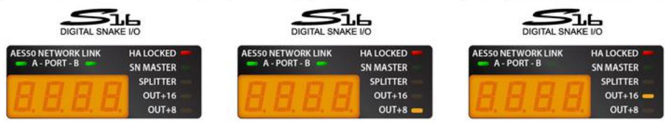
FOH console supplies clock synchronization and controls the S16 preamps exclusively (local HA control is blocked by console)
