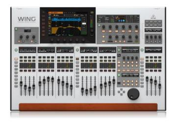
48-Channel, 28-Bus Full Stereo Digital Mixing Console with 24-Fader Control Surface and 10" Touch Screen
