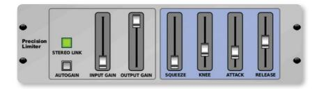
The **STEREO PRECISION LIMITER** is perfect for setting a precise volume limits, ensuring distortion-free and optimal signal integrity. Use the Stereo Precision Limiter to boost quiet signals or reduce the level of "hot" signals to prevent clipping. (Inspired by Sony Oxford Dynamics\*)
