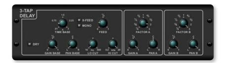
The **3-TAP DELAY** in the X32 COMPACT records the input signal and then echoes it back after a user-definable period of time and number of repeats. What makes the stereo and triple delay useful and outstanding is the linked tap-timing and musical choice of echo patterns.
