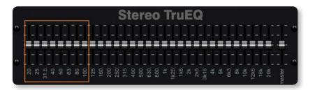
Our **TruEQ STEREO GEQ** delivers musical and responsive signal processing—perfect for general room equalization, indispensable for monitoring. X32 PRODUCER provides up to 16 mono graphic EQs, in addition to the multi-band parametric EQs in all channels and buses, to cope with the most demanding stage monitoring situation.
