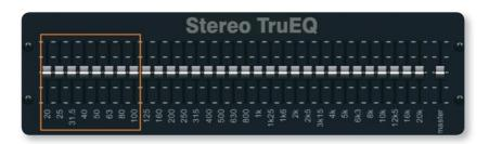
Our **TruEQ STEREO GEQ** delivers musical and responsive signal processing—perfect for general room equalization, indispensable for monitoring. X32 RACK provides up to 16 mono graphic EQs, in addition to the multi-band parametric EQs in all channels and buses, to cope with the most demanding stage monitoring situation.
