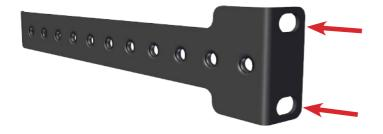
3. Screw the M6 mounting screw into the appropriate hole for both rear support brackets. Leave enough room between the head of the screw and rear bracket for the slotted end of the mounting brackets.
