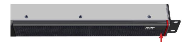
1. Begin by pressing the grille on the side that includes the amplifier type indicator text.
