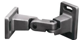
The LBC 1252/00 wall mounting bracket is for mounting loudspeakers directly onto a surface, such as a wall or ceiling. It is made from die-cast aluminum, and includes two lockable swivel joints to allow movement in two perpendicular planes for precise positioning.
