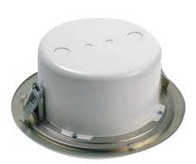
LBC 3099/41 with LBC 3082/00 fire dome assembly The unit has two built-in spring-loaded locking clamps to secure it into a hole in suspended ceilings and wallboards from 9 to 25 mm (0.35 to 1.0 in) thick. A circular template for marking a 210 mm (8.3 in) diameter hole is included with the loudspeaker.
