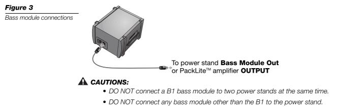
• Use only the supplied blue B1 bass module 4-wire cable to connect the B1 bass module to the power stand. The power stand uses the signals on two of the wires to automatically sense how many B1 bass modules are connected. DO NOT substitute the supplied cable with a 2-wire speaker cable.
