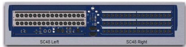
Detail of Devices tab indicating presence of two AO16 Cards output slots D and E
