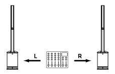
If you wish to run two POLAR 12s in stereo, route the mixing console's left channel to the system on the left and its right channel to the system on the right. Make sure the DSP settings for Mode, EQ, Delay, and so on are identical for both systems. See chapter 3 for more on this.
