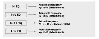
POLAR's three-band EQ serves to tune the system's overall sound. Hi EQ and Lo EQ are shelving filters; Mid EQ is semi-parametric.
