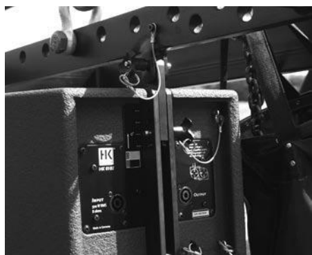
Figure 2: Mid/high enclosure with integrated flight attachments
