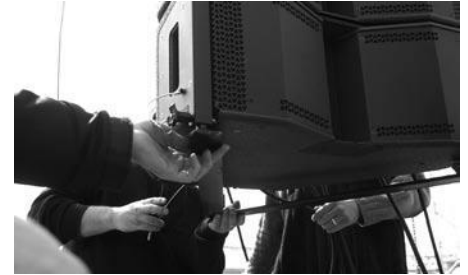
Figure 18: Mounting the bottom rigging frame
