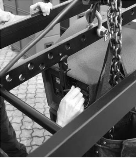
Figure 13: Mounting the top rigging frame
