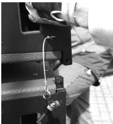
Figure 17 a: Mounting additional mid/high enclosures
