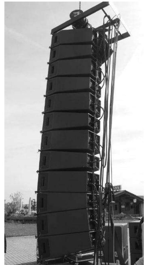
Figure 19: Attaching the lashing strap between the top and bottom rigging frames
