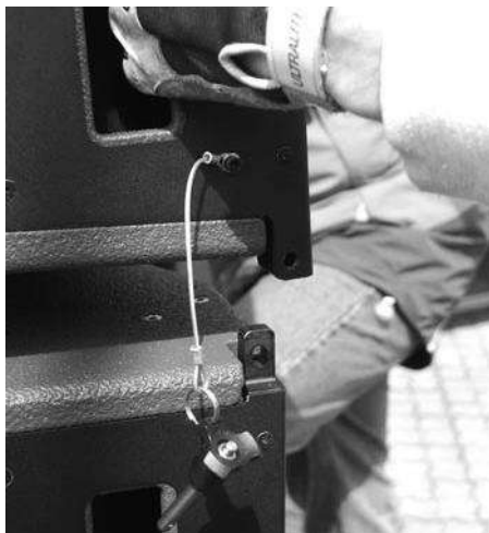
Figure 17 a: Mounting additional mid/high enclosures
