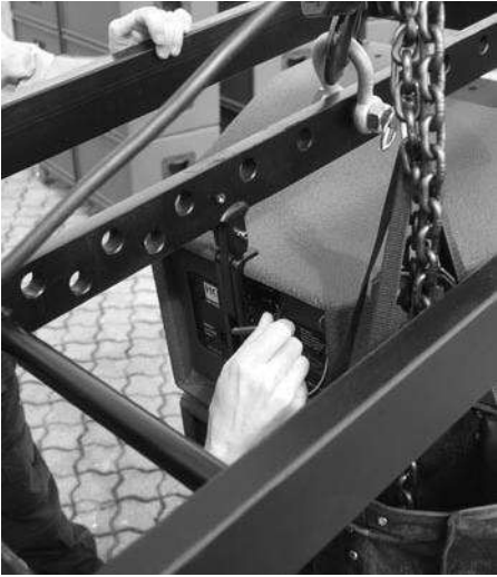
Figure 13: Mounting the top rigging frame
