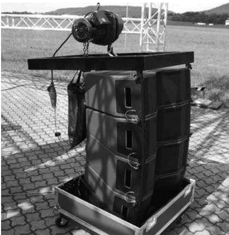
Figure 14: Mounting the main motor to the top rigging frame
