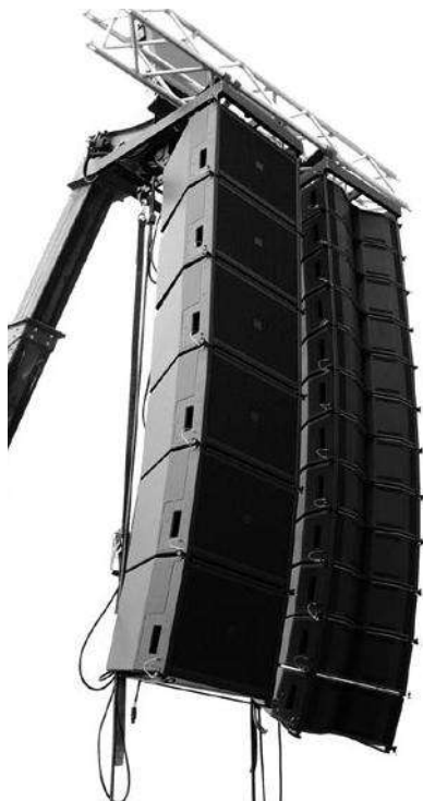
Figure 25: Flown CDR 210 F bass array next to a mid/high array
