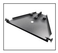
The ConTour Array™ stacking plate provides a base for connecting subwoofer and mid/high units. It screws onto the M20 pole mount. The variable tilt angle adjusts in 1.5° steps up to 9° max. The mid/high array is easily aligned by lightly rotating the stacking base plate on the subwoofer.
