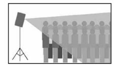
The HK AUDIO DuoTilt™ pole mount lets you align PREMIUM PR:O active cabinets along the horizontal plane to prevent or reduce troublesome ceiling reflections. The front aperture of the HK AUDIO DuoTilt™ provides a 3° angle, the rear aperture a 7° angle of tilt.
