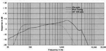
Frequency response of the 2204H in a closed box of 57 L  $(2~{\rm ft}^3)$  internal volume. Measured response of a typical production unit, including all peaks and dips, does not deviate more than 2 dB from the above curve. The dashed curve represents the response with a  $160~{\rm cm}^2~(25~{\rm in}^2)$  port,  $26~{\rm cm}~(10~{\rm in})$  long, tuning the enclosure to  $50~{\rm Hz}$ .
