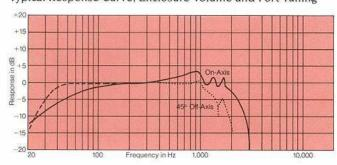
Frequency response contour of the 2235H taken in a hemispherical free-field environment, a closed box of 140 L (5 ft $^3$ ) internal volume enclosing the rear of the driver. Measured response of a typical production unit, including all peaks and dips, does not deviate more than 2 dB from the above curve. The dashed curve represents the response from a 160 cm $^2$  (25 in $^2$ ) port with a 28 cm (11 in) long duct tuning this enclosure to 30 Hz.
