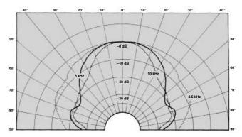
Polar response of the 2402H in the horizontal plane, measured with  $\frac{1}{2}$ -octave band pink noise in a free-field environment. The curves were traced by an automatic recorder. Power fed to the 2402H was adjusted to provide the same 0 dB reference for each curve.
