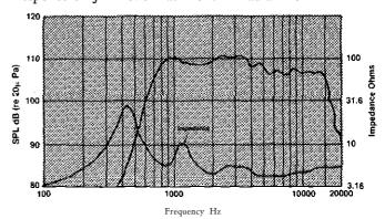
Frequency response of the 2426H coupled to a JBL 2370 Flat-Front Bi-Radial horn, measured on-axis at a distance of 1 meter with a 1 watt (2.83 V RMS) input in a reflection-free environment, with impedance vs. frequency curve. The increased high-frequency output is due to the horn design s increasing directivity in the vertical plan.
