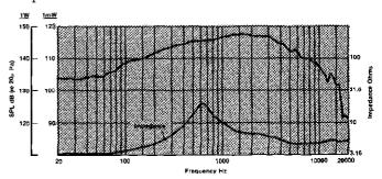
Frequency response and impedance modulus of Model 2426H coupled to a 25 mm (1 in) diameter terminated plane-wave tube. This is the power response of the transducer, and is the frequent) response that will be obtained on a true full-bandwidth constantdirectivity horn design, such as JBL s 2360 series of Constant Coverage Bi-Radial Horns.
