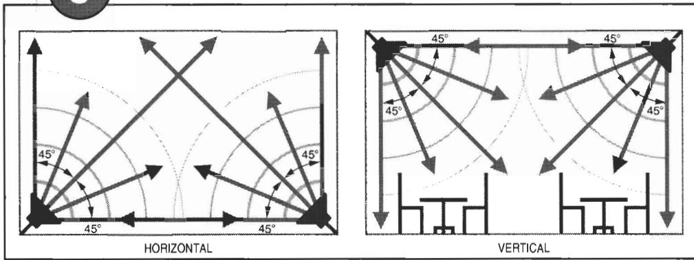
**• High Frequency Coverage** - High frequencies go where you point them. Simply aim the center axis of the speaker into the plane slightly above the listening area. The  $90^\circ \times 90^\circ$  horns of the Control® Contractor Series disperse the high notes by  $45^\circ$  off axis in every direction. For large or unusually shaped rooms, divide the area into zones and let the horn patterns dictate the spacing between the speakers (see diag. 5).
