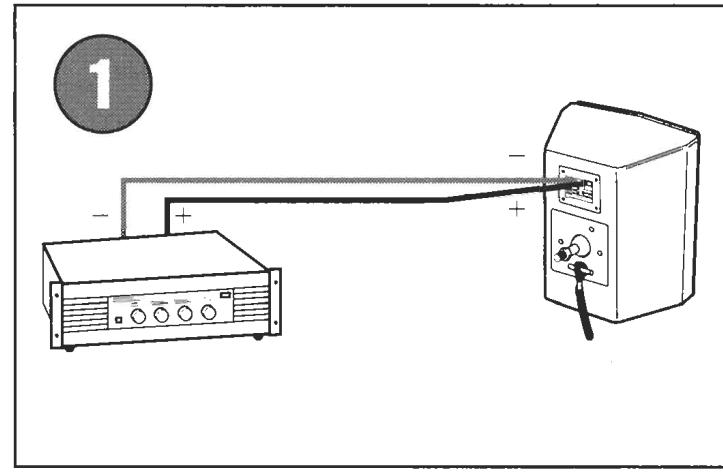
**8Ω each** - Since the loudspeakers have a rated impedance of 8Ω each, more than one speaker may usually be wired to one amplifier channel (see diag. 2). (See "amplifier impedance load" below.)
