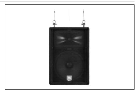
The JRX112Mi is an economical, suspendable, twelve-inch, two-way speaker system designed for installation where ground stacking or pole mounting is impractical or undesirable. The JRX112Mi is well suited to a variety of sound reinforcement applications including live music, music playback and speech. Other than the substitution of three, threaded M10 suspension points for the handles, feet and pole-mount, the JRX112Mi is identical to the popular JRX112M portable sound reinforcement speaker.
