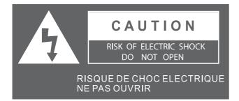
The lightning flash with arrowhead symbol within an equilateral triangle, is intended to alert the user to the presence of uninsulated. "Dangerous Voltage" within the products enclosure that may be of sufficient magnitude to consitute a risk of electric shock to persons.
