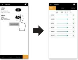
3. Three pages are available for setting the input gain, input level and output level respectively: touch the top menu buttons according to the needed adjustment.
