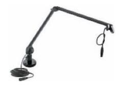
This exclusive microphone arm with a 3/8" or 5/8" thread connector in a modern design with a new innovative table clamp for quick and easy positioning of a microphone in the studio or at a multimedia work station. The 6 m long internally guided microphone cable has a 3 pin XLR plug connector. Microphones to max. 1.5 kg are easily held in any position.
