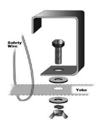
**NOTE:** Use washers\* and spring washers\* when attaching your hook clamp\* to the yoke 1. For installation of the hook clamp\* and safety wire\*.
