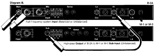
For increased flexibility, however, you may prefer to retain separate control of the bi-amplified and subwoofer system levels. To do so, you should connect your
