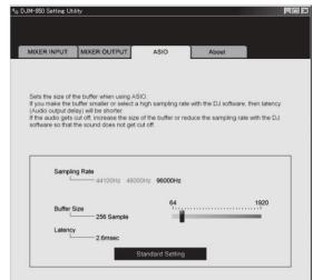
If the buffer size is made large, drops in audio data (breaks in the sound) occur less easily, but the time lag due to the delay in the transfer of the audio data (latency) increases.
