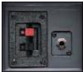
Input terminals Parallel 1/4 TRS phone jack and push wire-type input terminals.
