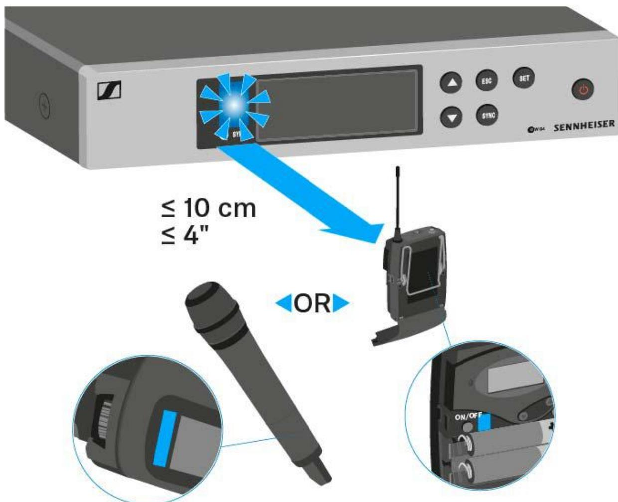
The parameters are transferred to the transmitter. The blue LED blinks during transmission.
