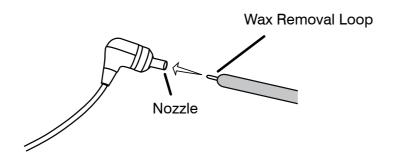
When cleaning, do not force any object through the earphone nozzle! This will damage the earphone sound filter.
