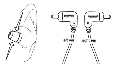
To change earphone sleeve, twist and pull sleeve to remove it from the nozzle. Push new sleeve onto nozzle until you feel it slide completely over barb. If any part of the nozzle is exposed, sleeve is not properly installed. Replace sleeves if they do not grip the nozzle tightly.
