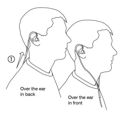
Tighten the cable and take up slack by raising the cable sleeve (1).
