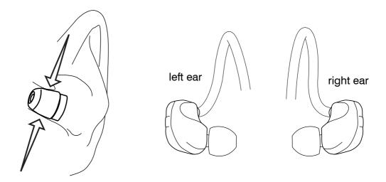
Make sure that the sleeve completely covers the earphone nozzle. If any part of the nozzle is exposed, the sleeve is not properly installed.
