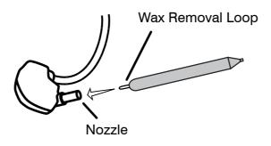
When cleaning, do not force any object through the earphone nozzle! This will damage the earphone sound filter.
