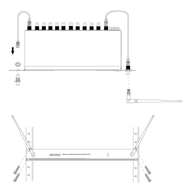
Installation and Cable Connections
