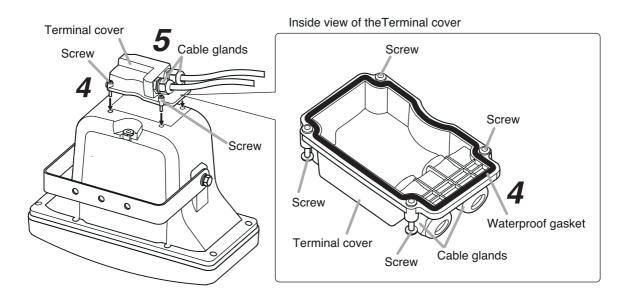
Step 7. Securely tighten the cable glands.
