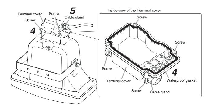
Step 5. Securely tighten the cable gland.
