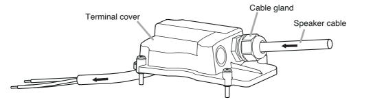
Step 3. Connect the speaker cable according to the polarity indication at the screw terminal.
