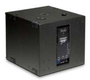
It consists of one 15" reflex-loaded low frequency driver in an optimally tuned enclosure with pole mount socket and moulded corner mouldings constructed from 18mm (3/4") birch plywood and incorporating an integrated Class D amplifier and control electronics module. The rear panel carries input and link XLRs, RJ485 network connectors, low frequency contour, power switch and status LED's.
