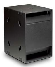
It consists of a single 18" bandpass-loaded low frequency driver in an optimally tuned 18mm (3/4") birch plywood enclosure with pole mount socket constructed from with a built-in pole mount socket and moulded corner protectors. Two Speakon NL4 connectors provide input and link out connections.
