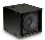
It consists of a single 15" reflex-loaded low frequency driver in an optimally tuned 18mm (3/4") birch plywood enclosure with built-in pole mount socket and moulded corner protectors. Two Speakon NL4 connectors provide input and link out connections.
