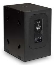
It consists of one 18" bandpass-loaded low frequency driver in an optimally tuned enclosure with pole mount socket and moulded corner protaectors constructed from 18mm (3/4") birch plywood and incorporating an integrated Class D amplifier and control electronics module. He rear panel carries input and link XLRs, RJ485 network connectors, low frequency contour, power switch and status LED's.
