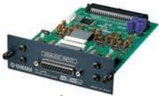
MY8-AD96 8 channel Analog Input Card
