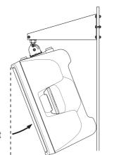
The tilt angle depends on the position relation between the speaker and the wall. The maximum downward tilt angle is shown in the following chart.
