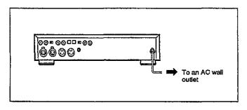
After connecting all equipment, connect the AC power cord plug to an AC wall outlet.
