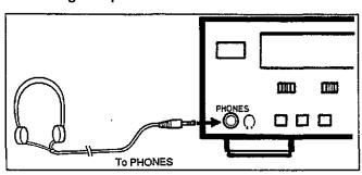
For best results, use 8-ohm to 32-ohm headphones with a standard stereo headphone plug 1/4" (6.3 mm). The headphone volume can be adjusted with the PHONES LEVEL control.
