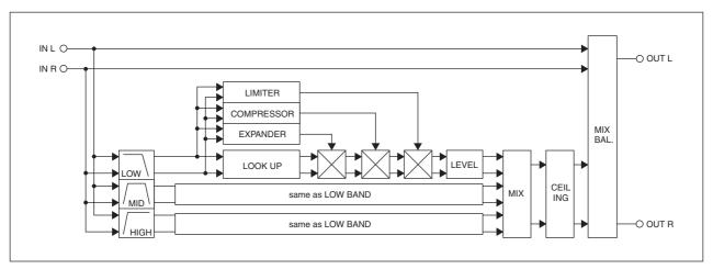
This effect splits the signal into three frequency bands, and individually controls the dynamic range of each band. It lets you use three types of processor — a compressor, expander, and limiter — in combination. The signal is sent through the expander, compressor, and limiter in that order.
