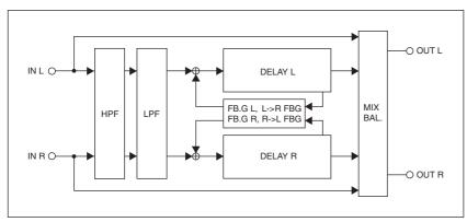
These effects add two delays; one each to the L and R channels. This is similar to Stereo Delay (page 40), but Echo mixes the L/R channel delay sounds for feedback. You can specify the amount of feedback sent from the L channel to the R channel, and from the R channel to the L channel.
