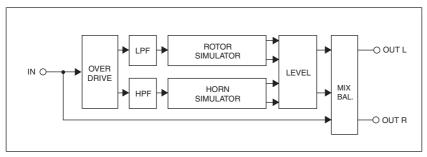
This effect simulates a rotary speaker. A rotary speaker physically turns its internal speaker and horn to produce a Doppler effect, giving a distinctive character to the sound.
