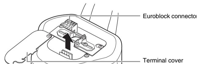
3 After loosening the terminal screws of the Euroblock connector with a flat-blade screwdriver, insert the cable into each terminal and tighten the screws. Make sure that cables cannot be pulled out.
