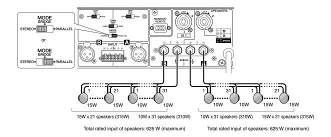
The **XP3500** enables you to connect in **bridge fashion** multiple high-impedance speakers that support **100V** line output. You can connect speakers with a total rated input of up to **625 W**.
