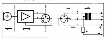
Input circuit incorporating transformer without center tap (ungrounded).
