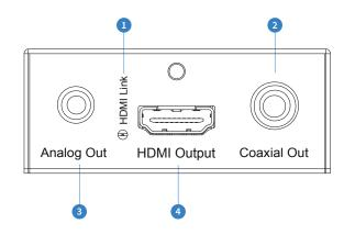
1 HDMI LED indicator - Lit when detecting a HDMI 3 L/R Out Analogue Audio Out - Extracted audio from HDMI connection to a display/end point. input (Compatible with 2ch PCM only).
