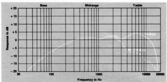
Frequency response contour of the 8110H taken in a hemispherical free-field environment. Measured response of a typical production unit, including all peaks and dips, does not deviate more than 4 dB from the above curve. Additional acoustic loading will further extend bass response.
